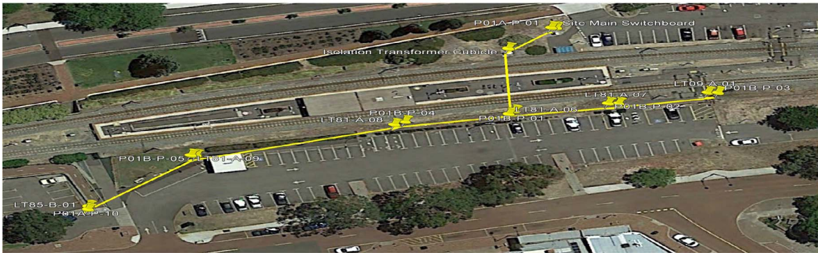
Fig. 12. Circuit of power distribution from the SMSB.
