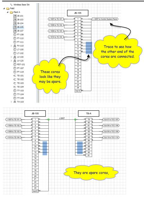
Finding spare cores is usually a lengthy exercise of accessing drawings and then comparing the cores shown on them with the total number of cores available in the cable. Often then there will have to be a site inspection as well. It may take many days to find (or fail to find) spare cores which as you have just seen can be found pretty well instantaneously with DAD.
