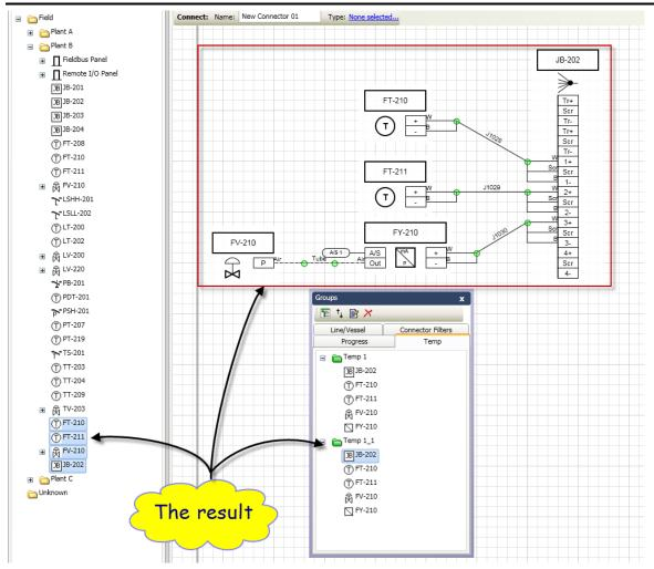
Maybe needs a warning to rename components to avoid duplicates as no "\_1" suffix is added automatically as per other cloning.
