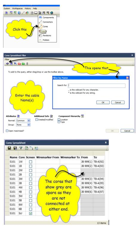
Or as is often the case you are looking for spare cores terminated on a device, this is how you do it:
