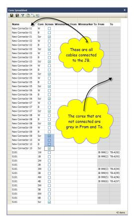
This second set shows how to find where the spare cores are connected at both ends. In this case you must decide which cores are spare by inspection of the connections:
